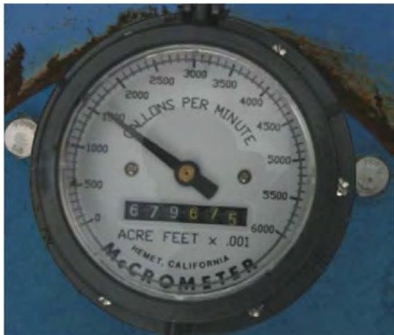
Figure 3: Example Flow Meter Display (Totalizer reads 679.675 acre-feet)
