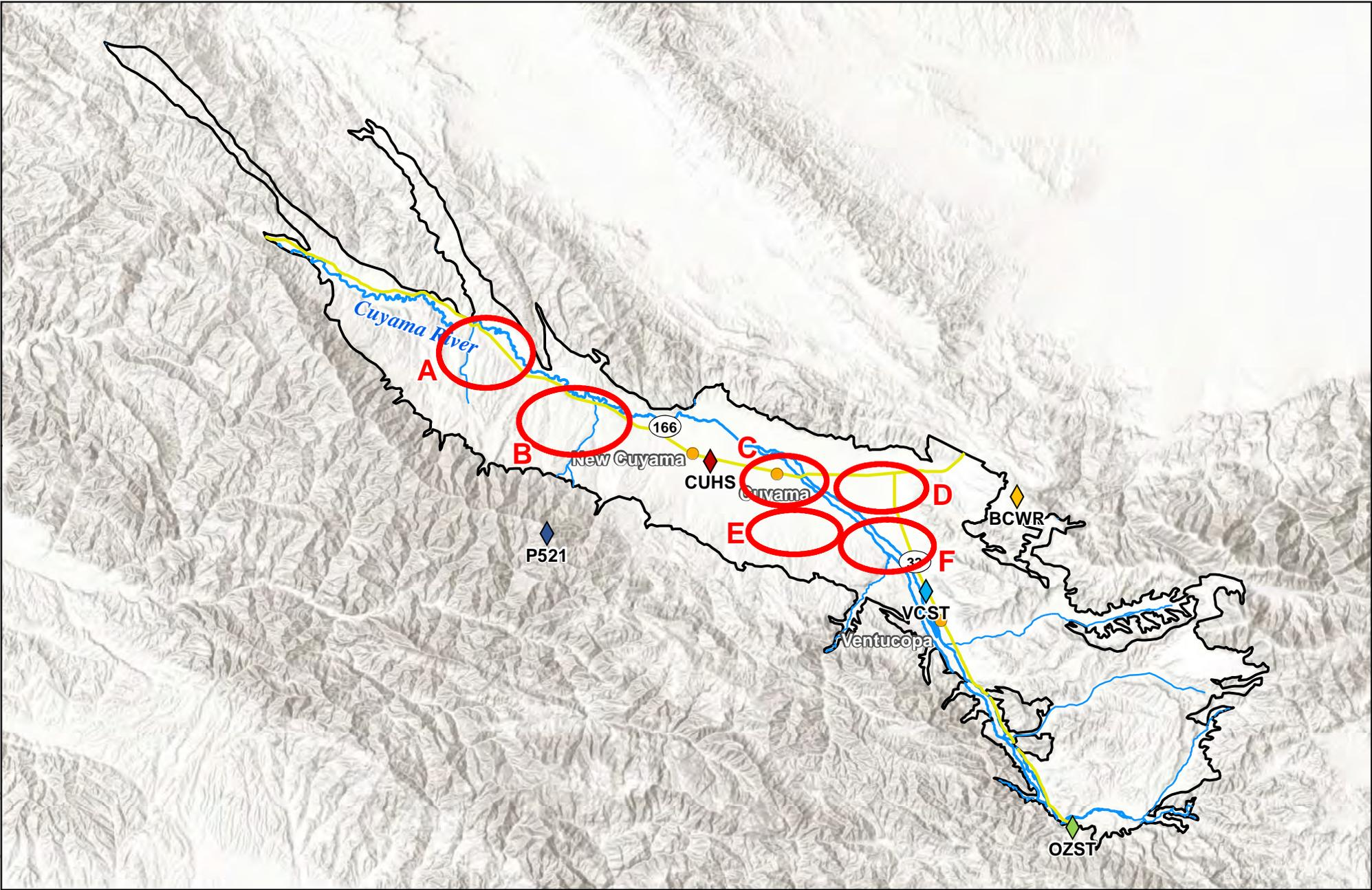
**Figure 4-23: Subsidence Monitoring Location Data Gap Areas**
