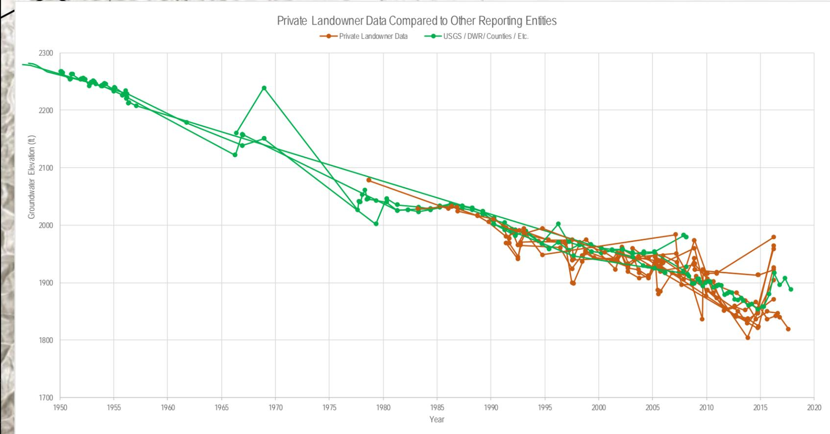
**Figure 2-27: Central Cuyama GW Basin Wells and Hydrographs by Data Source**
