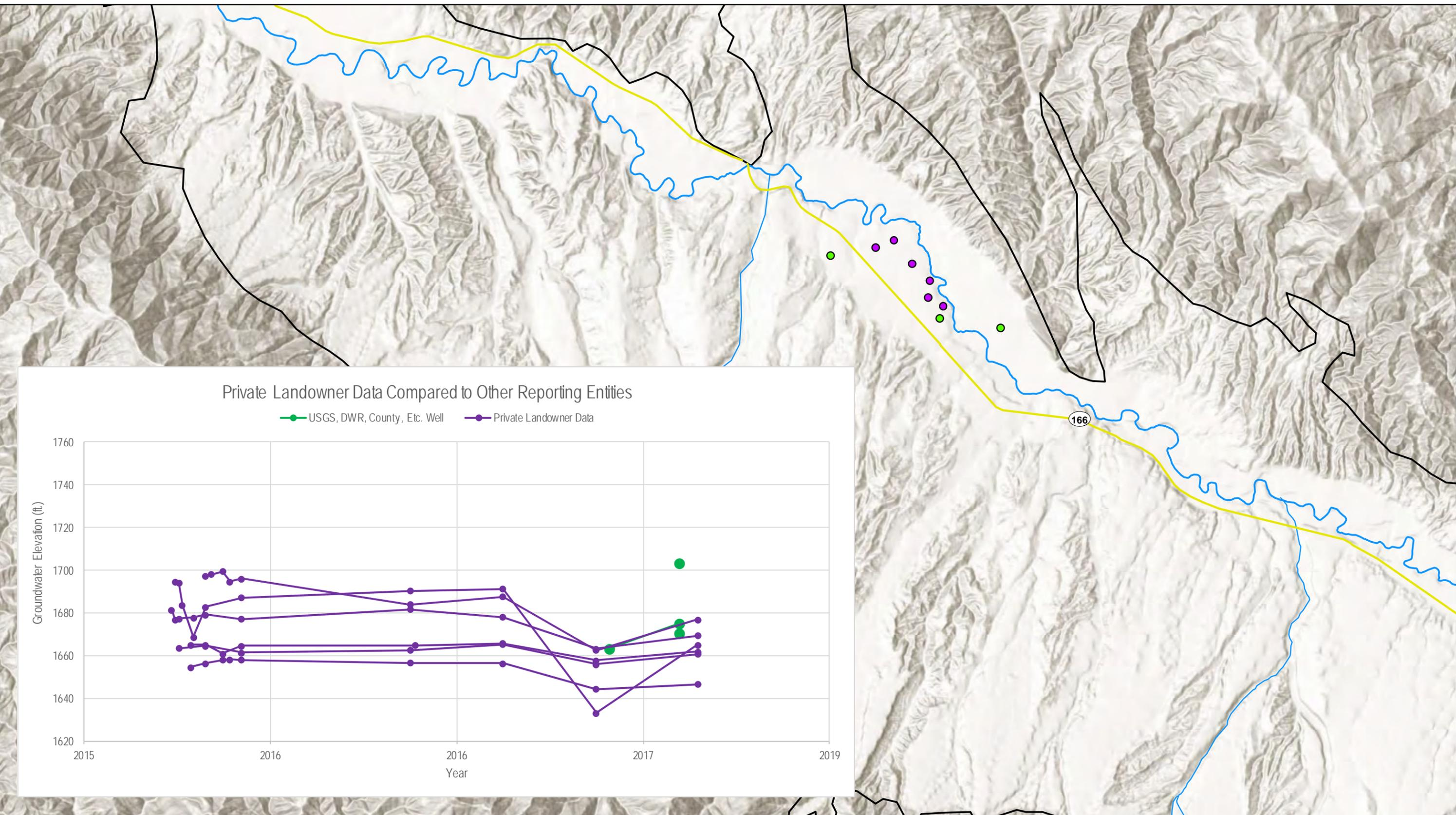
**Figure 2-28: Western Cuyama GW Basin Wells and Hydrographs by Data Source**
