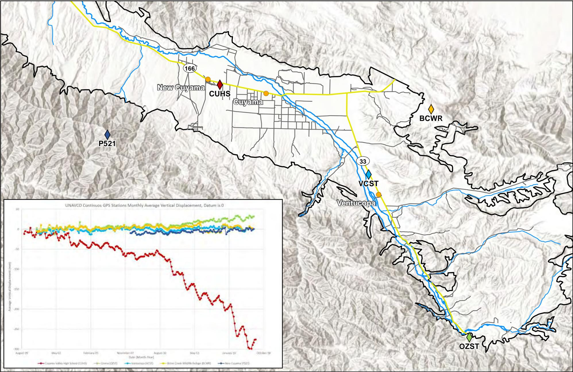
**Figure 5-4: Cuyama GW Basin Subsidence Monitoring Locations**
